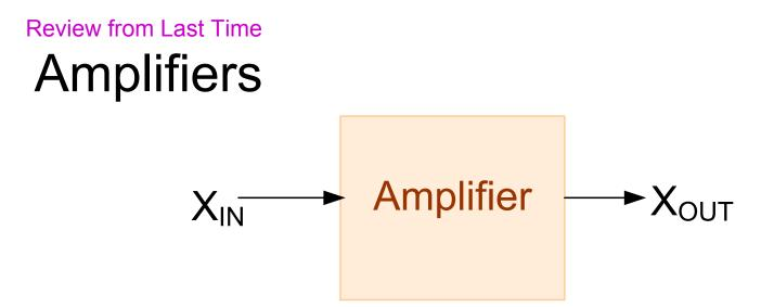
An ideal amplifier is linear and has a frequency independent transfer function that does not change with source or load impedance
