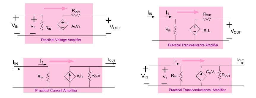
When nonideal, the functional form of all four basic amplifiers are identical and they differ only in the value of the model parameters
