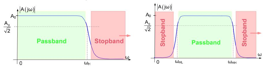
The passband is the frequency range over which an amplifier passes or amplifies signals and the stopband is the frequency range where signals are attenuated
