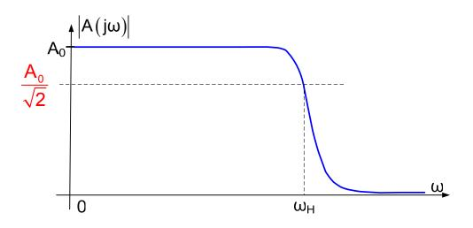
Claim: The half-power frequency is the frequency where the magnitude of the voltage gain drops to  $\frac{A_0}{\sqrt{2}}$  where  $A_0$  is the maximum gain
