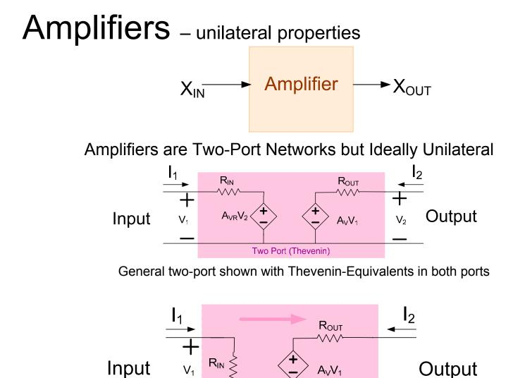
Signals propagate in only one direction in unilateral circuits
