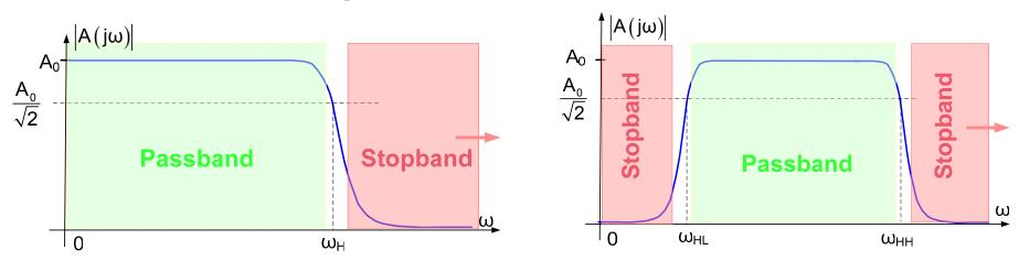
Definition: The amplifier bandwidth is the width of the "passband" of the amplifier
